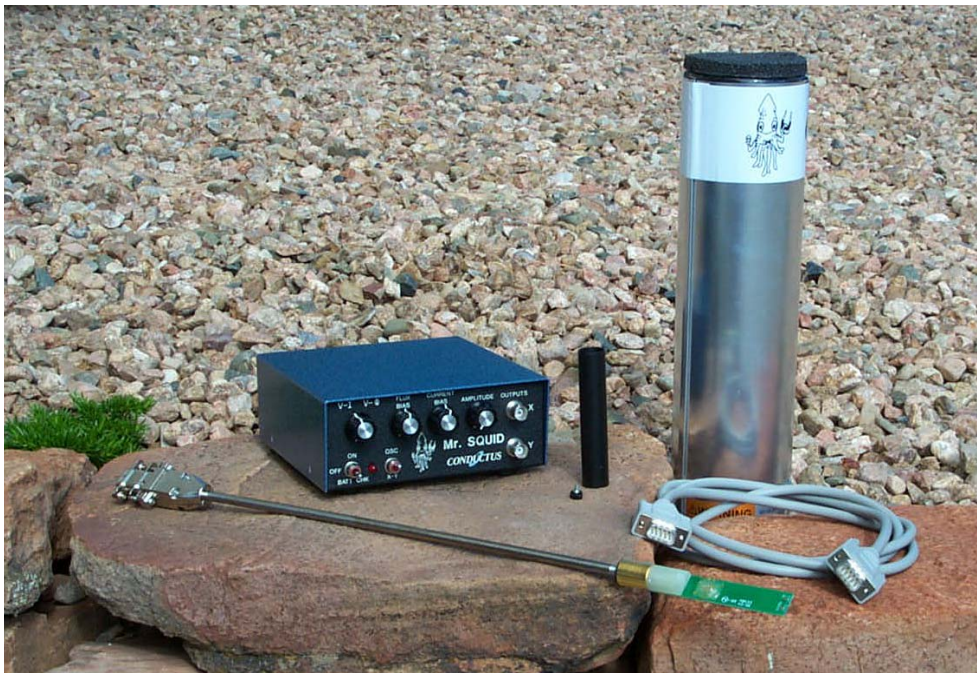
Figure 2-1 Mr. SQUID® system components.
