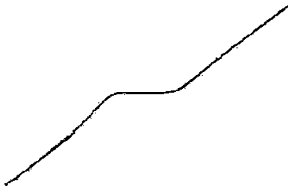
Figure 5-4 A typical Mr. SQUID ® V-I characteristic.
