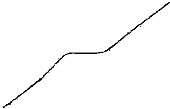
Figure 3-3 Typical Mr. SQUID ® V-I characteristic.
