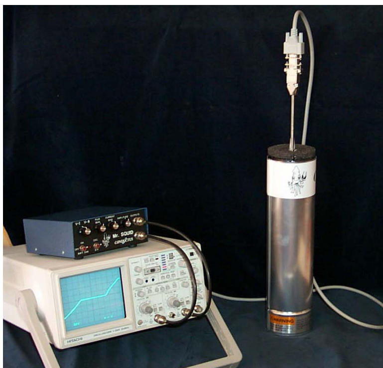
Figure 2-5 An operating Mr. SQUID ® system using an oscilloscope display.
